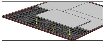
Lay the foam mats next to each other jointless; if necessary, cut individual pieces to fit
