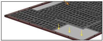
Install the lower mats jointless throughout the whole area; if necessary, cut the mats to fit
