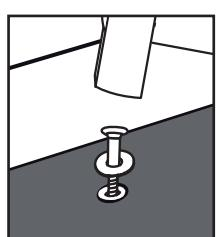
pound in anchors and washers until they are seated firmly and are slightly countersunk
