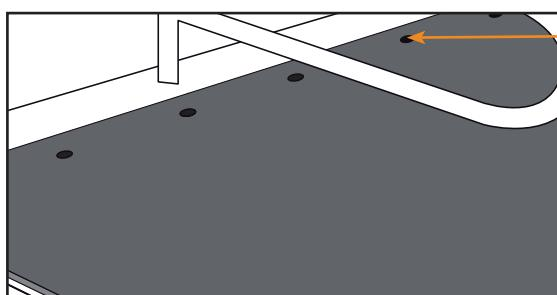
fasten at the front edge through the predrilled holes
